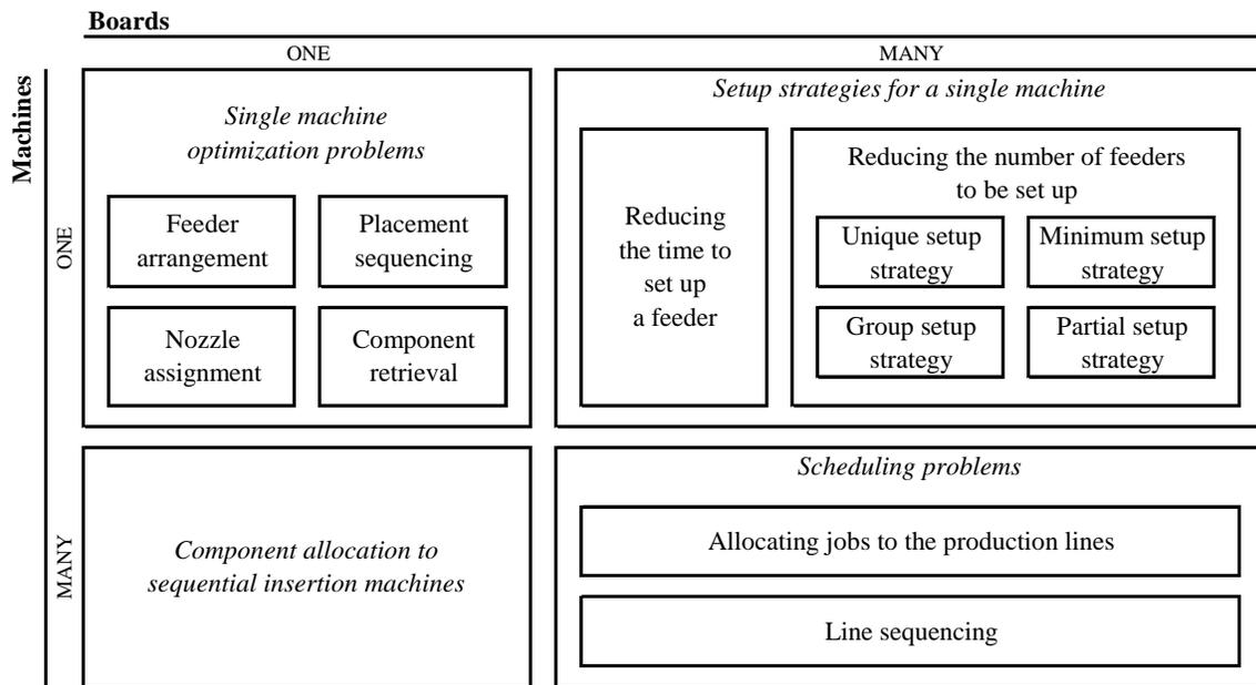
Figure 1: A hierarchical classification scheme of the PCB assembly problems
